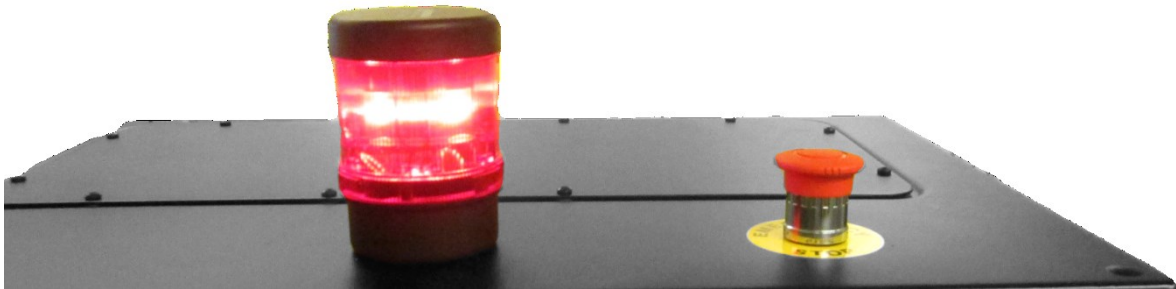
Figure 5 An active warning light means the lasers are powered.
