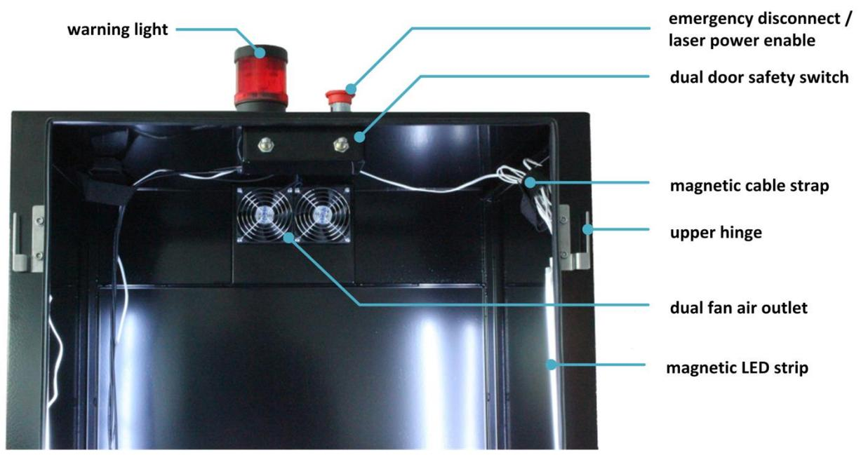
Figure 8 Safety Box interior - roof area
