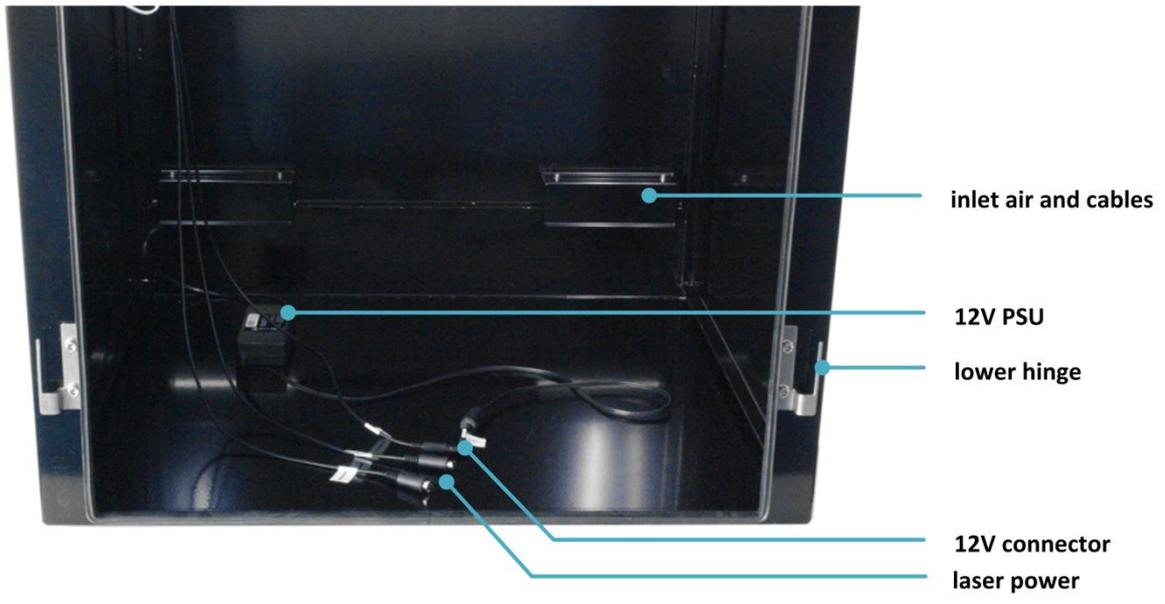
Figure 7 Safety Box 2 interior - bottom area.
