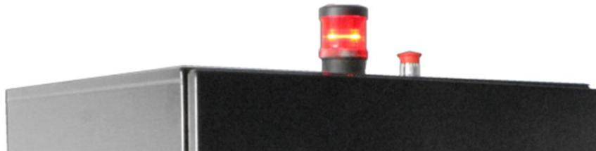
*Figure 5 An active warning light means the lasers are electrically powered.*
