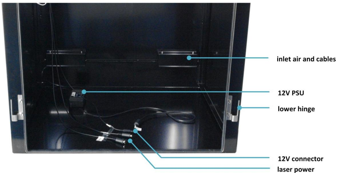
*Figure 2 Inlet of the power cable to the PSU.*
